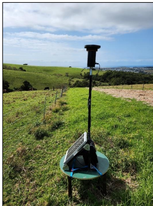
N2 – SiteHive Continuous real time noise monitor in operation
