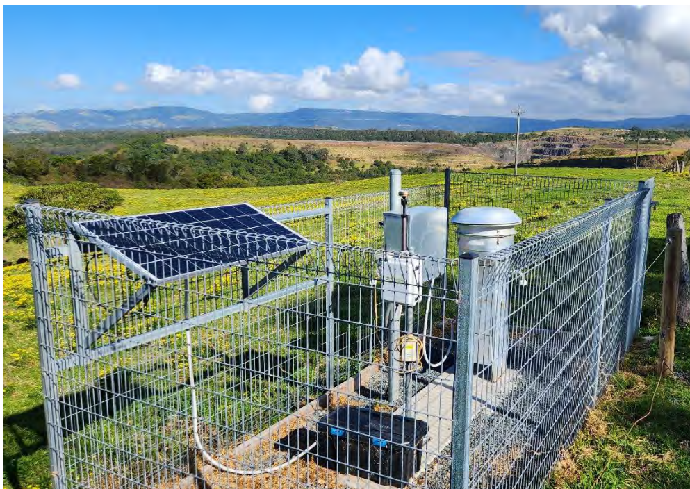
A1 and A2 – Continuous real time particulate monitor (front) and HVAS (back)
