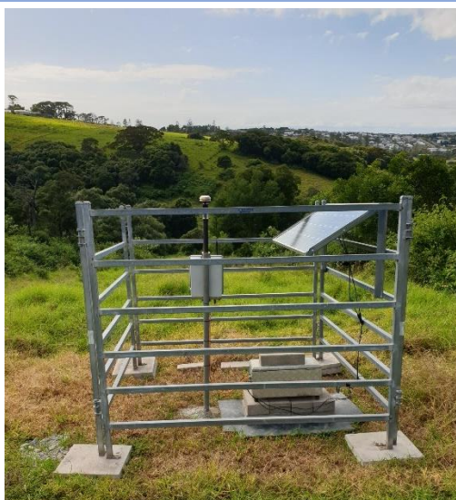
APD4 – Continuous real time particulate monitor in operation
