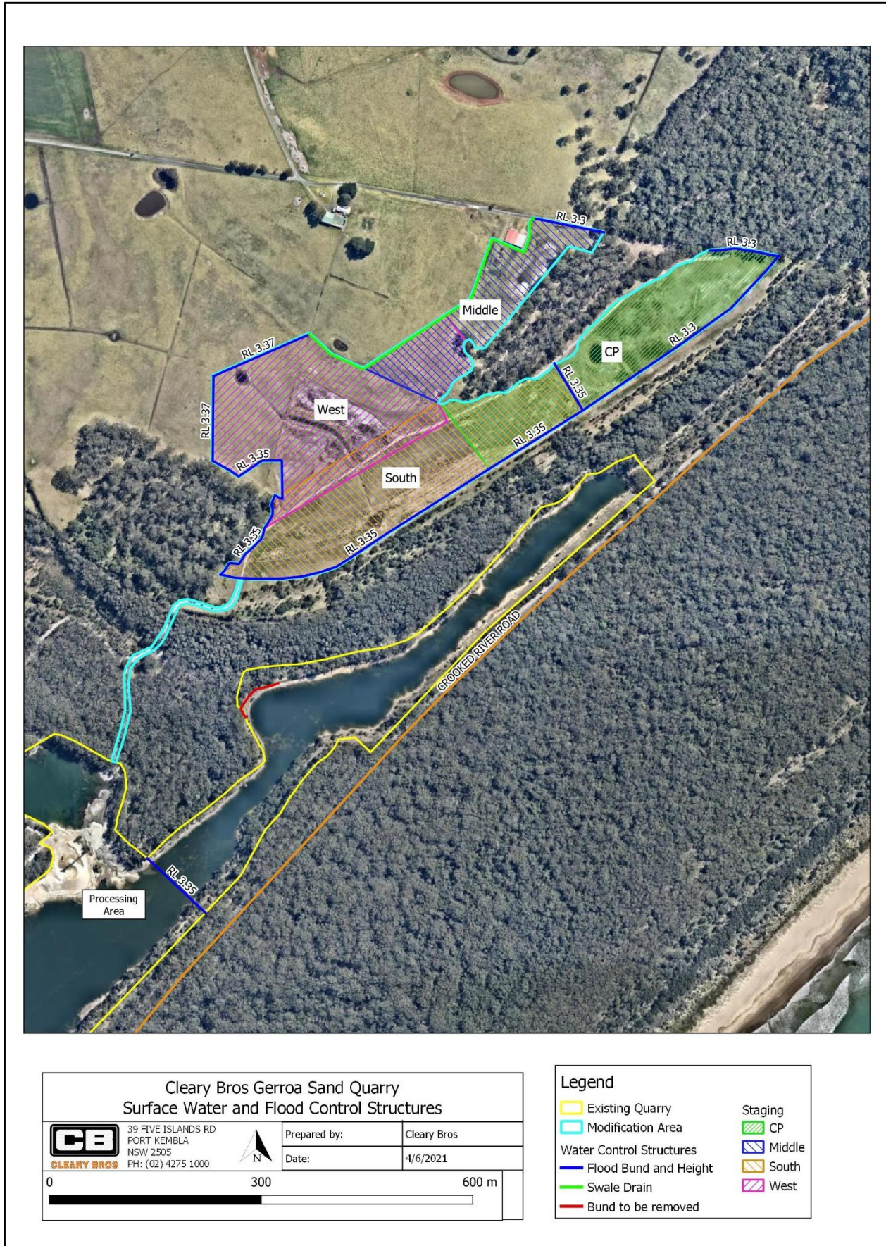
Figure 2-3 Surface Water and Flood Control Structures
