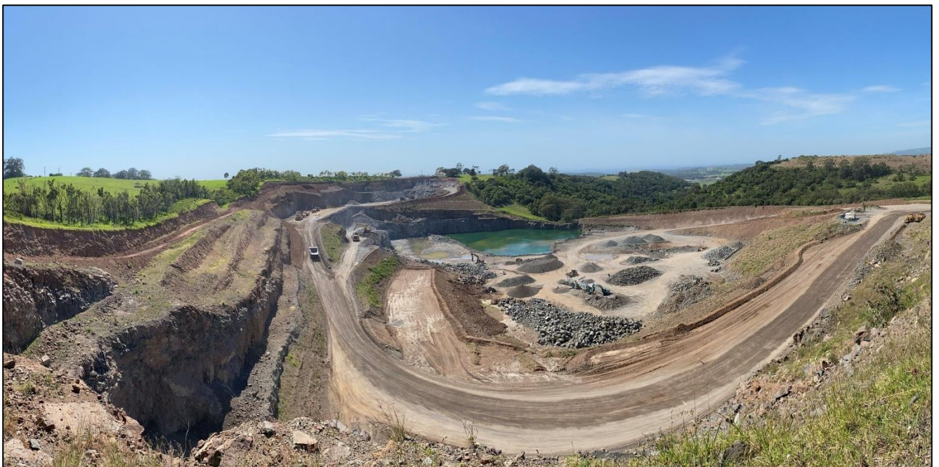
Figure 3.13b: View looking north east, showing extraction area with relatively larger sump that has transitioned to east (16/12/2019)
