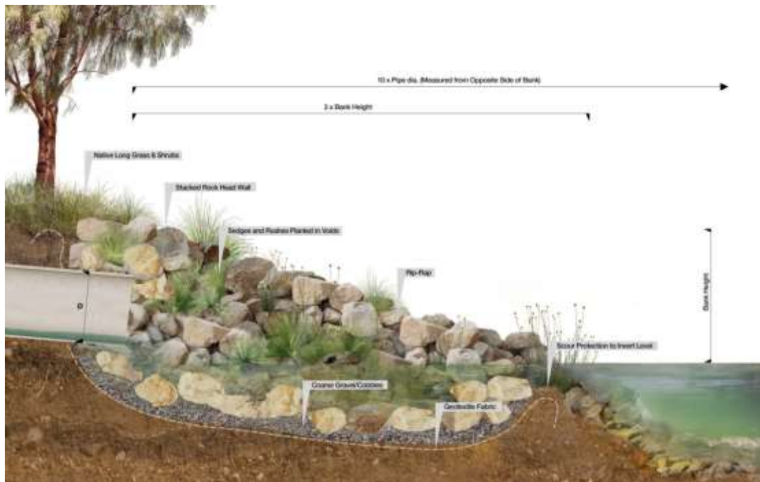
Figure 6: Headwall setback (Sydney Water, 2014)
